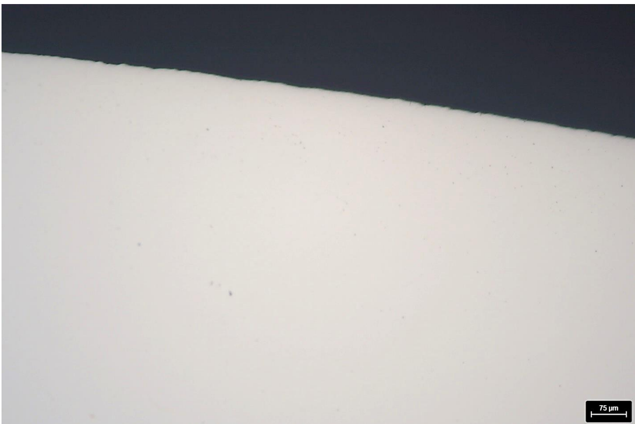
Figure 13: The outer diameter of "MRA" ring sample before etching – 100 x.
