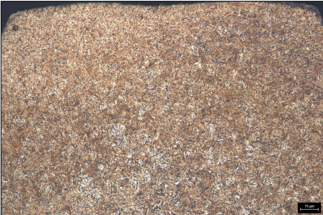
Figure 10: The microstructure after etching with 3% nitric acid – 100 x.
