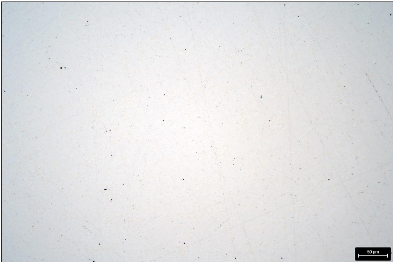
Figure 10: Sample 2585_15_OF4 after polishing step with GAMMA and 3 µm – 200 x
