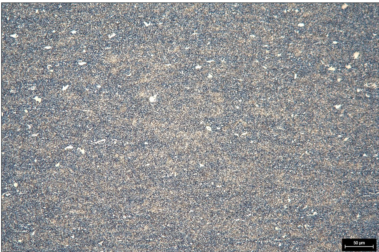
Figure 7: Sample 2493_25 after etching with NITAL – 200 x
