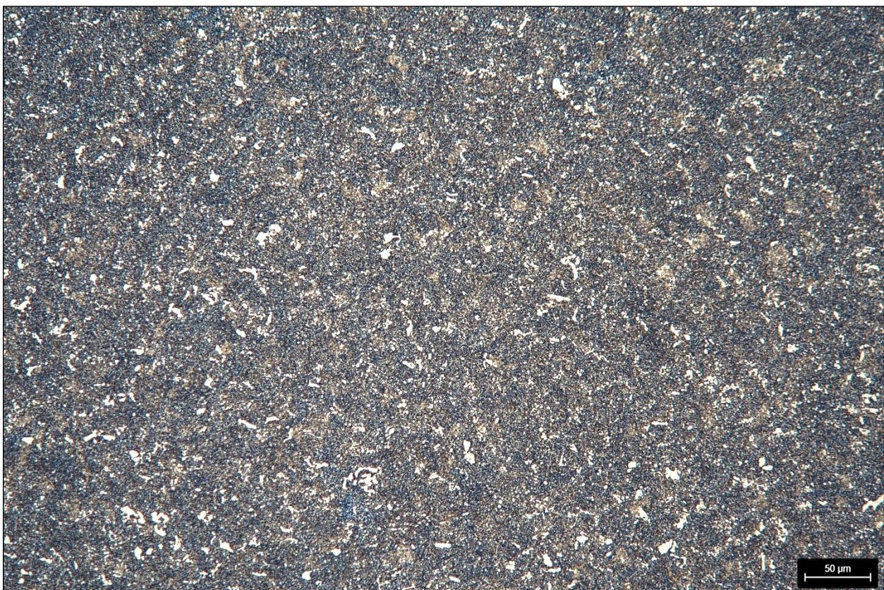
Figure 9: Sample 2585_15_OF4 after etching with NITAL – 200 x
