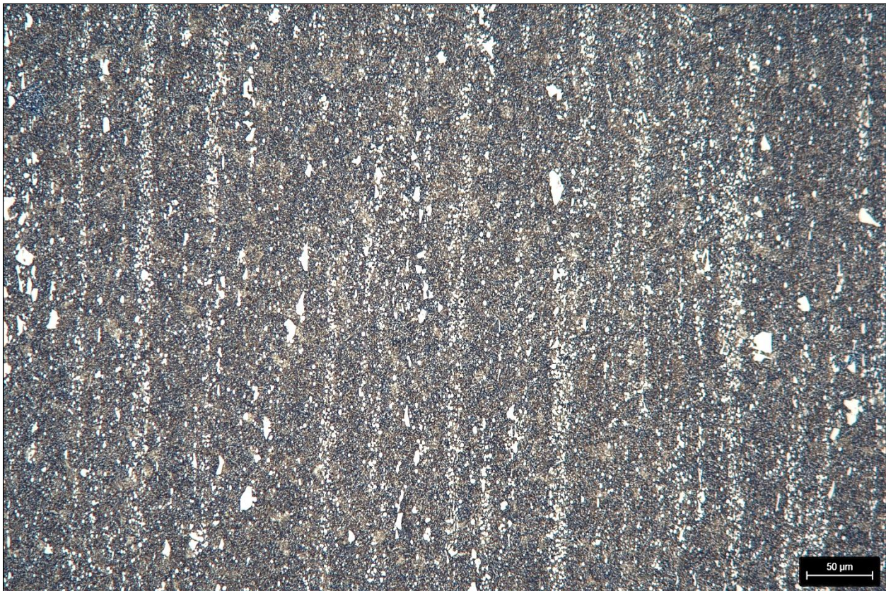
Figure 8: Sample 2493_13 after etching with NITAL – 200 x
