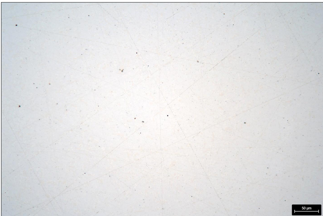
Figure 11: Sample 2493_12 after polishing step with GAMMA and 3 µm – 200 x
