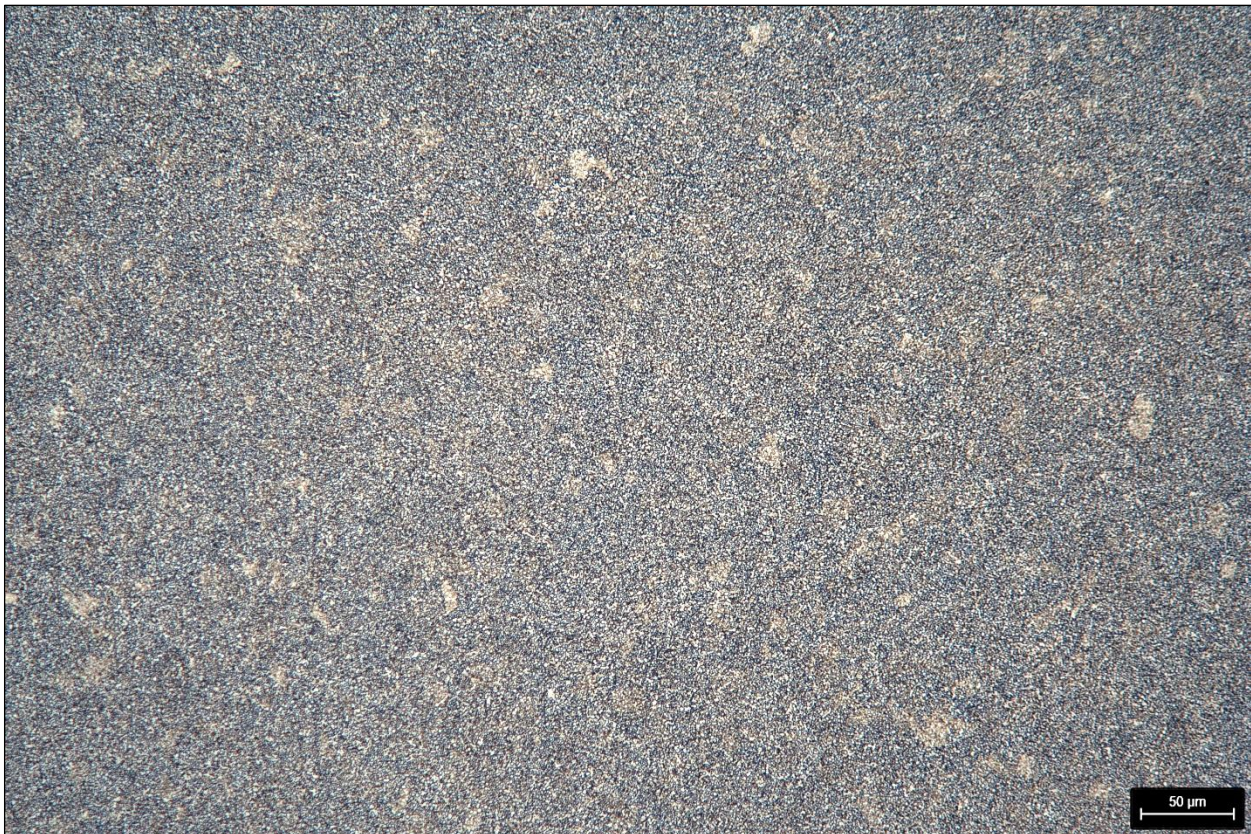
Figure 4: Sample 2485_43_OF4 after etching with NITAL – 200 x
