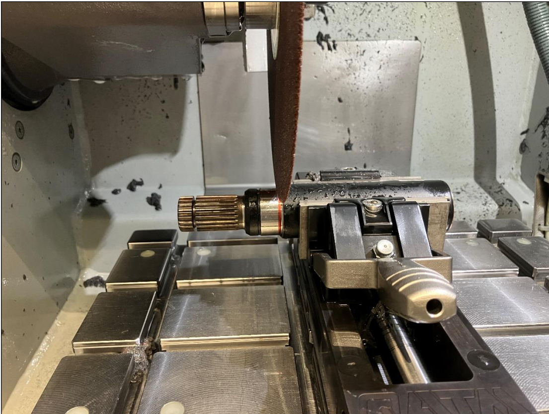
Figure 8: Cutting position 2 – BEFORE cutting process (Qtool 80 with 2x prism jaw 40 mm).
