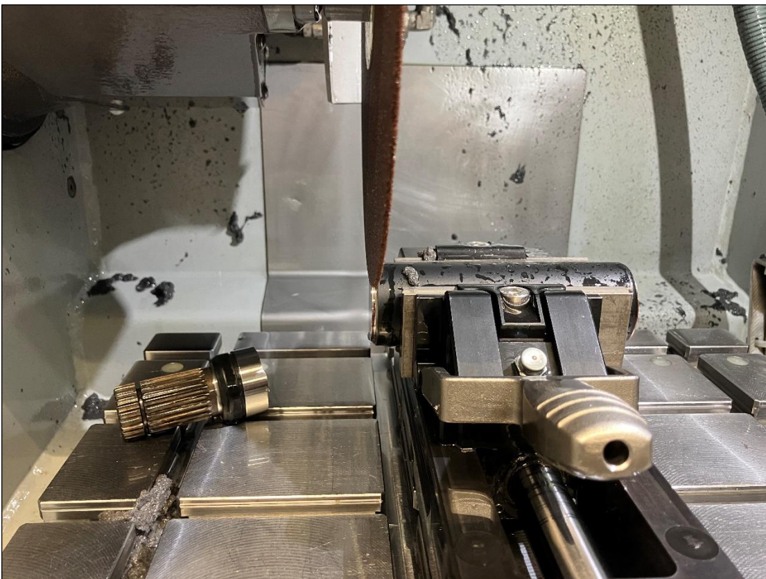
Figure 9: Cutting position 2 – AFTER cutting process (automatic vertical cut with Y-Axis).
