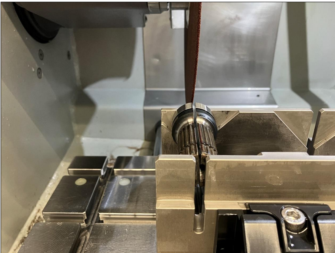
Figure 13: Cutting position 4 – AFTER cutting process (automatic horizontal cut with X-Axis).
