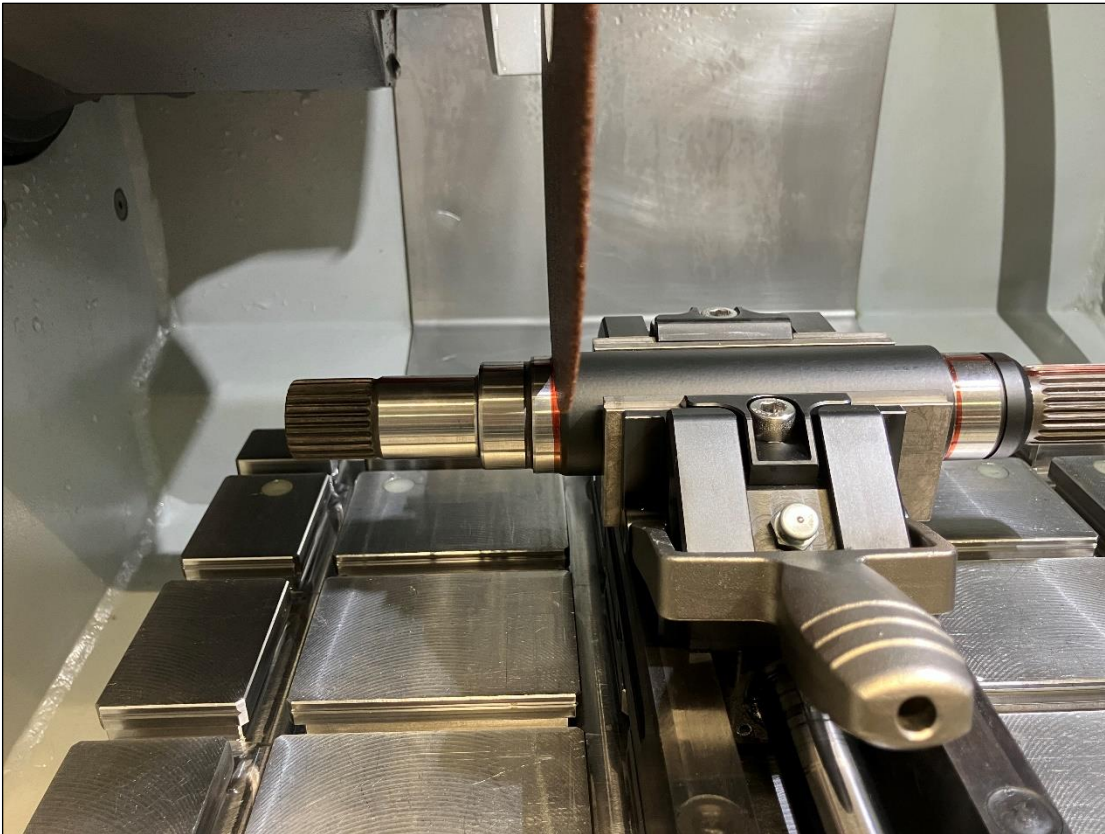
Figure 6: Cutting position 1 – BEFORE cutting process (Qtool 80 with 2x prism jaw 40 mm).
