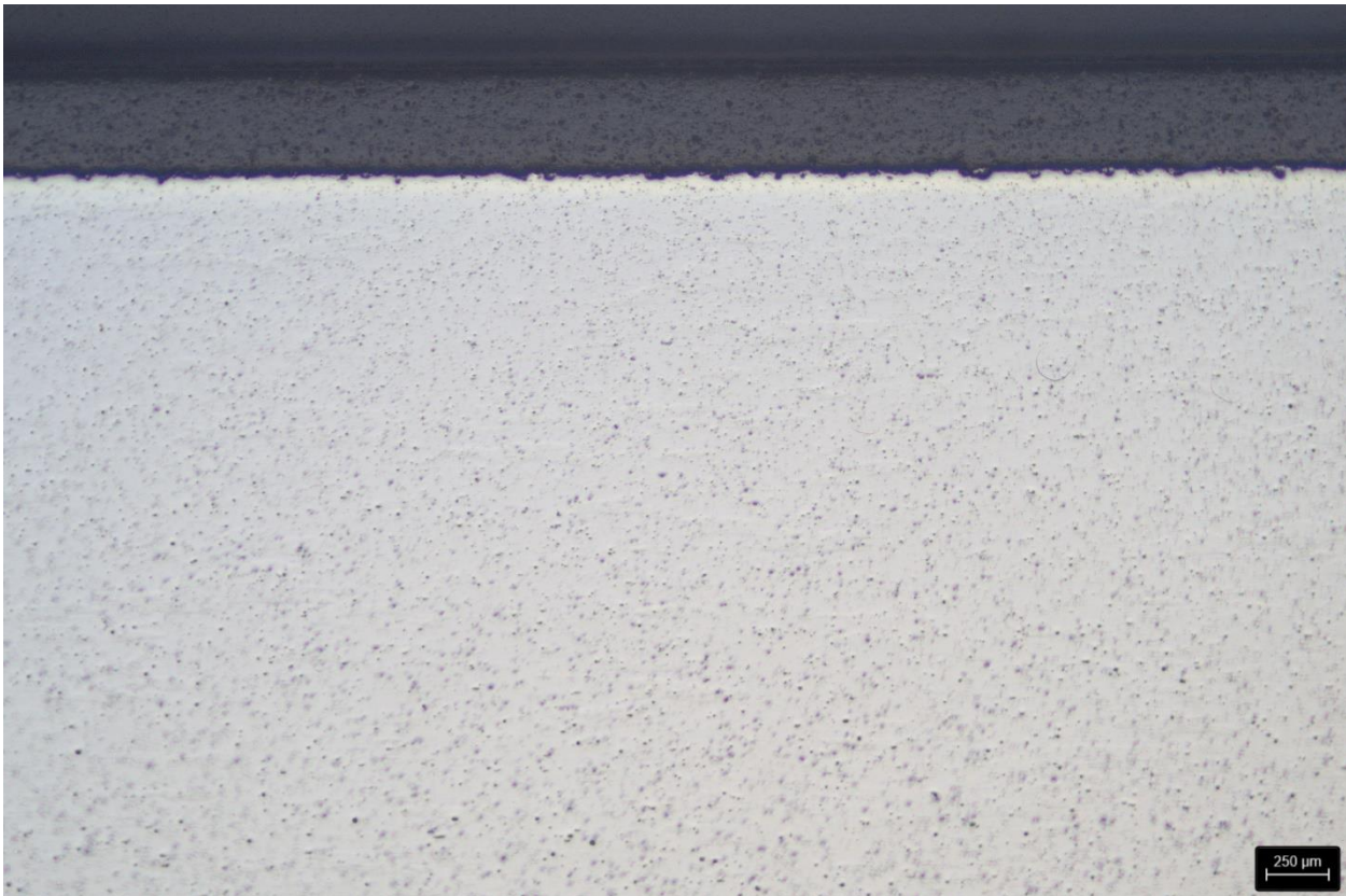
Figure 11: Ceramic sample after mounting with UV 55. No gap has been detected – 25 x
