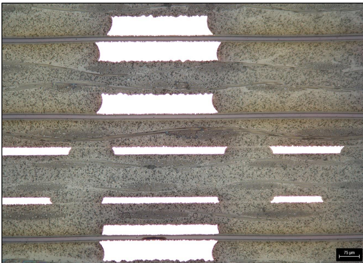
Figure 8: The CFRP in the PCB part – 100 x
