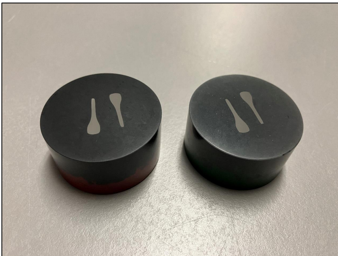
Figure 3: Samples after hot mounting with Qpress 50 ( \varnothing 40 mm).
