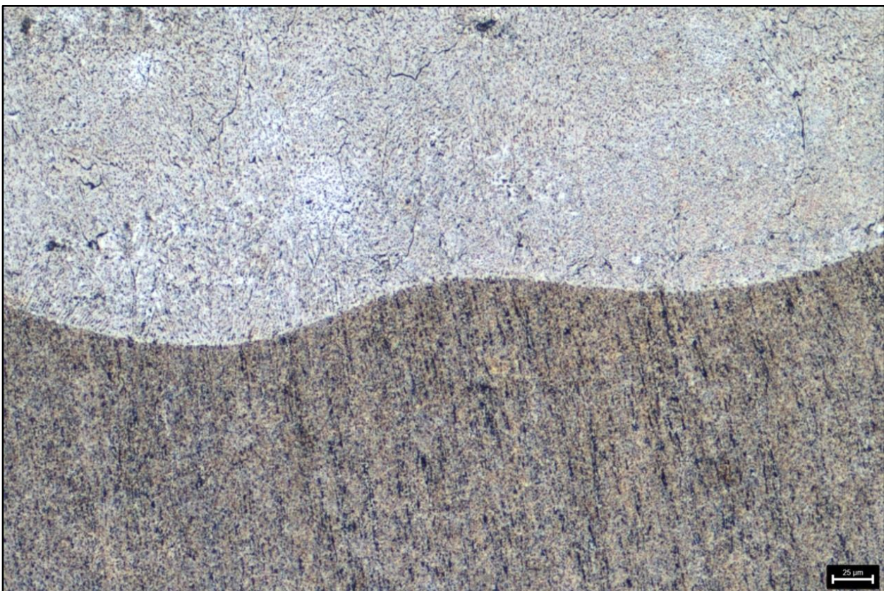
Figure 9: Welding seam - Sodium hydroxide - Transition to sheet 2 - 200x.
