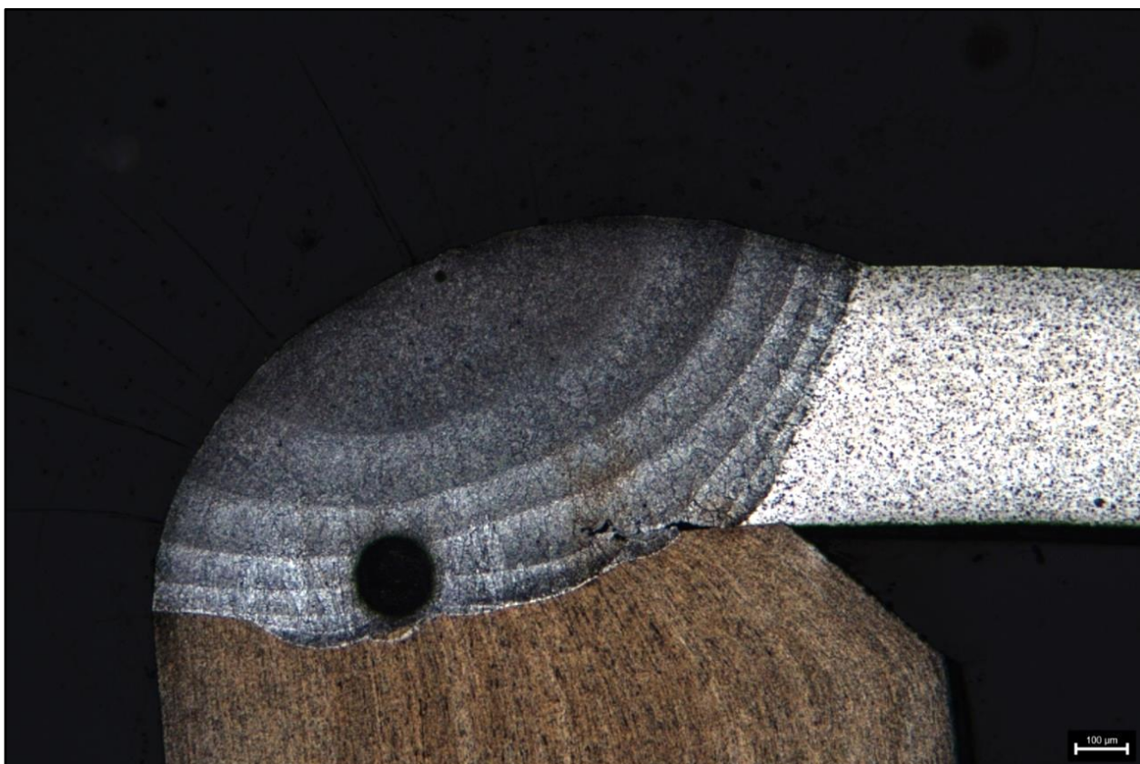
Figure 15: Welding seam - Kroll - 50x.
