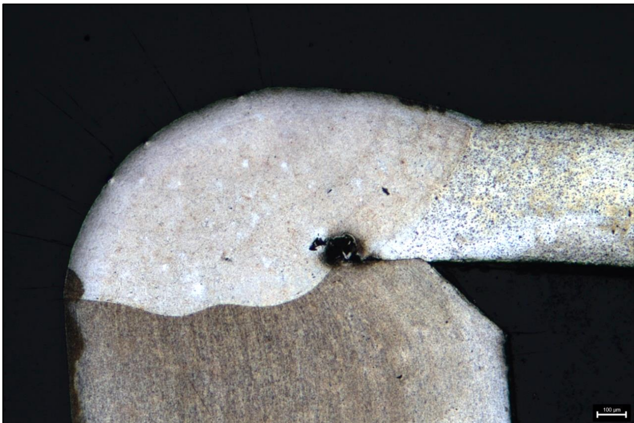
Figure 7: Welding seam - Sodium hydroxide - 50x.
