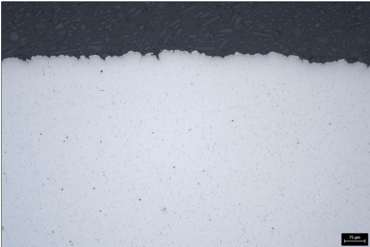
Abb. 6: Probe 2257 – 1.2.1. – Epo schwarz - Qpol 250 A1 – Rand - 100x.
