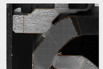
Test point pattern on a non-bedded specimen
