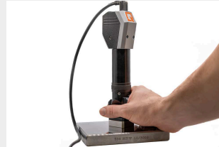
INDIRECT CALIBRATION USING A HARDNESS TEST BLOCK
