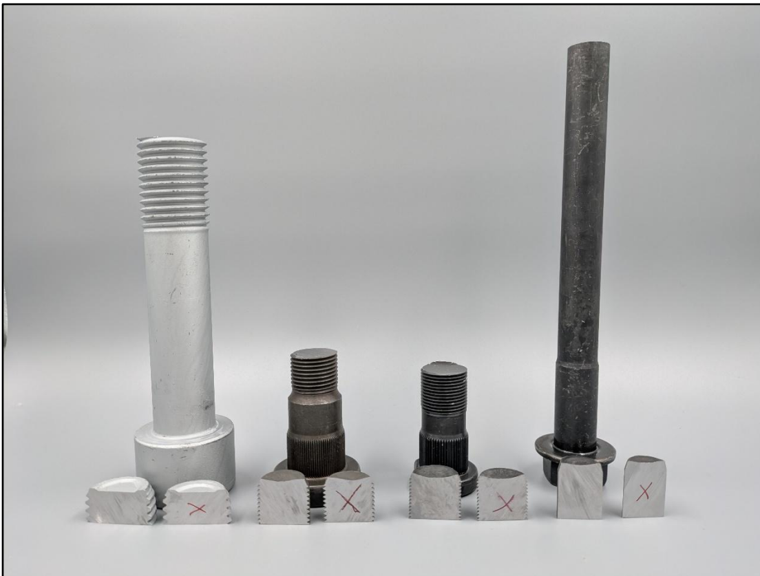
Figure 7. Overview sample after cutting
