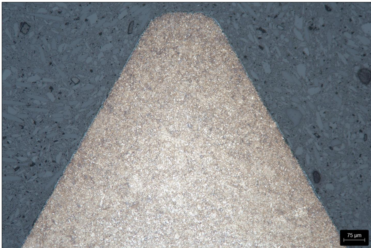
Figure 13. Crest of the thread profile of sample - 100:1
