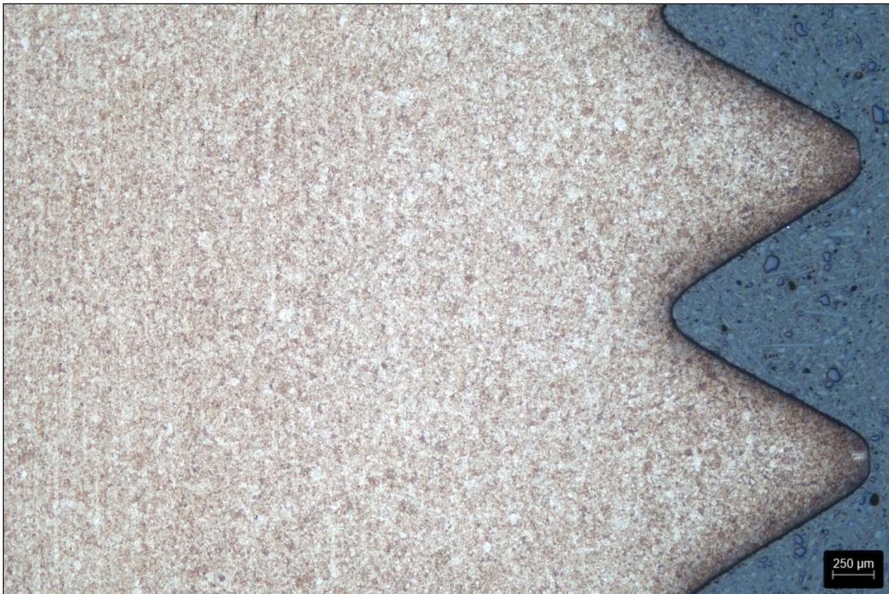
Figure 11. Overview of the thread profile - 25:1
